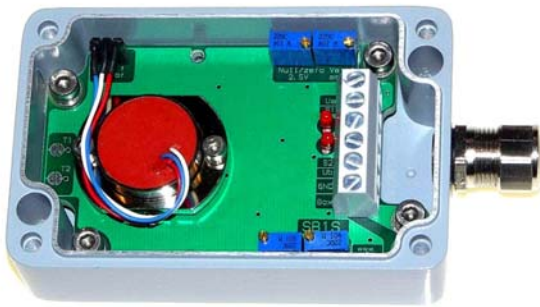
Sensor box containing one sensor, one signal conditioner with 0...5V output and two open-collector output switches
