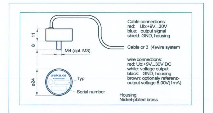
Attention! These sensors are not suited for applications subject to high mechanical shocks! Due to the sensor type the NB is sensitive to shock!
